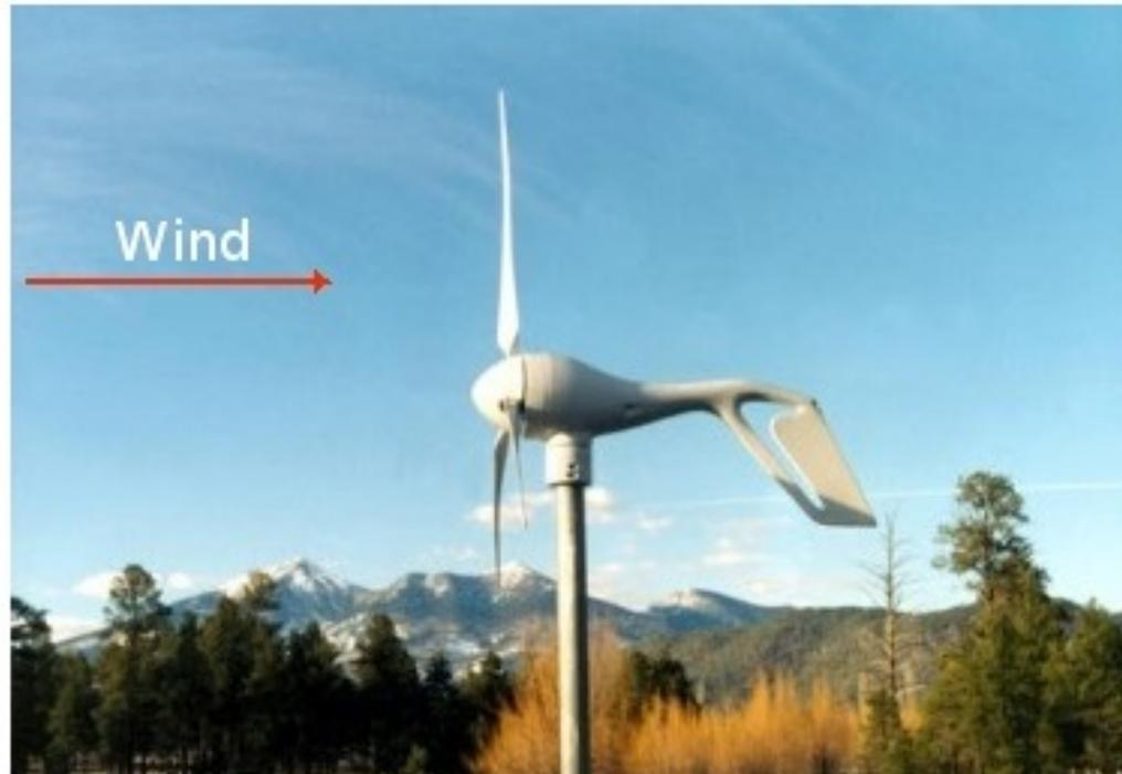
**Advantage** The reduced tower shading. The air will start to bend around the tower before it passes it so there is some loss of power from the interference, just not the degree as in the downwind turbine.
