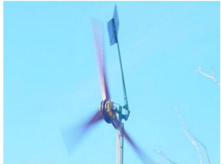
This photo shows a home-built 17-foot diameter 3.5 kW turbine with the tail in fully furling position. The machine is still making near maximum power, but it facing at an angle into the wind to reduce wind input.
