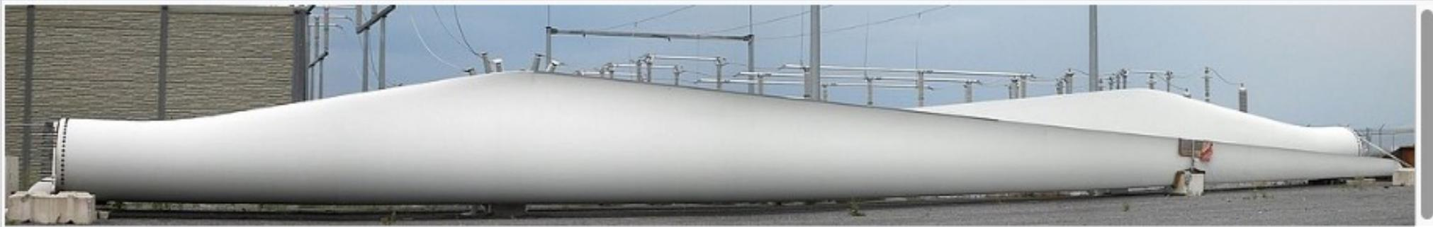
Fiberglass-reinforced epoxy blades of Siemens SWT-2.3-101 wind turbines. The blade size of 49 meters<sup>[45]</sup> is in comparison to a substation behind them at Wolfe Island Wind Farm.
